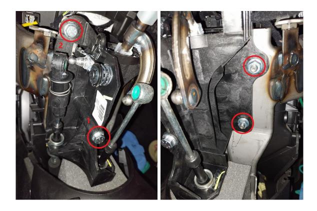
**10** - Before installing the PS shifter assembly, loosen the circled screws to facilitate the installation of the cables.
