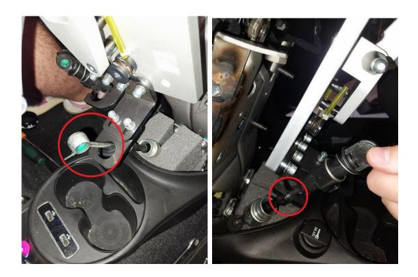
**12** - Position the supplied washer behind the shifter assembly on the top left screw (see step 9), then proceed with installing the 4 screws. (**Note** - Replace the original long screw with the one supplied in the pack).
