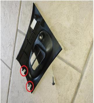
**2** - Remove the passenger's side tunnel cover by unscrewing the screw and releasing the 2 clips on the back.
