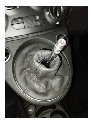
**4** – Lift the boot and cut the zip tie, then remove the boot by pulling it upwards.
