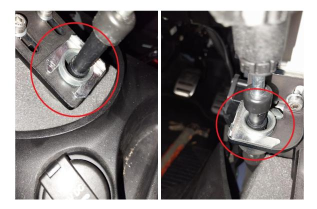
14 - Grease the ball-head pins and insert them into the cable ends. (Note – Before reconnecting the cables, check that the gearbox is in neutral)
