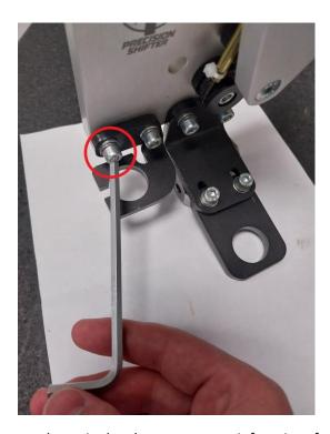
(Note – Tighten the circled screw as shown in the photo to prevent it from interfering with the connected cable)
