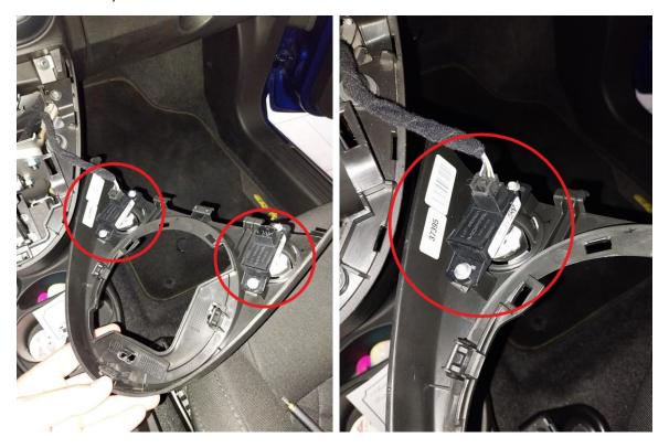
**6** - Unscrew the fixing screws (the ones circled) and remove the central cover.
