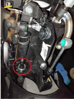
**9** - Unscrew the fixing screws and remove the original shifter assembly.
